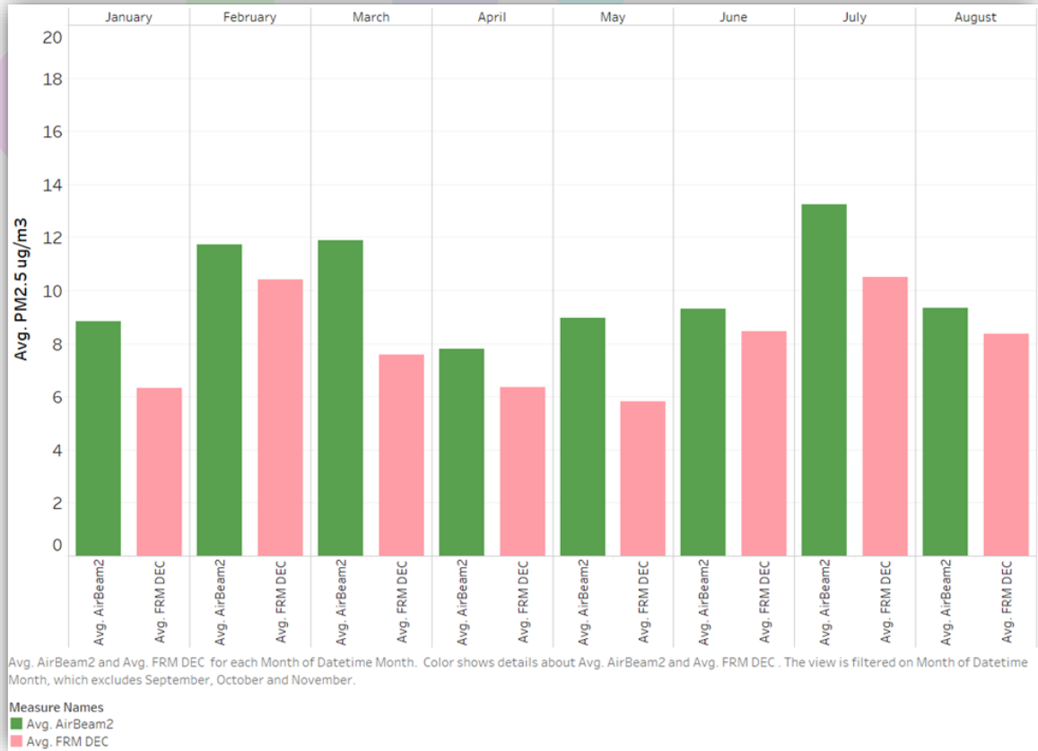
Fig.21. Monthly average of PM 2.5 concentrations for AirBeam2 and FRM for a period of January to August 2019.
