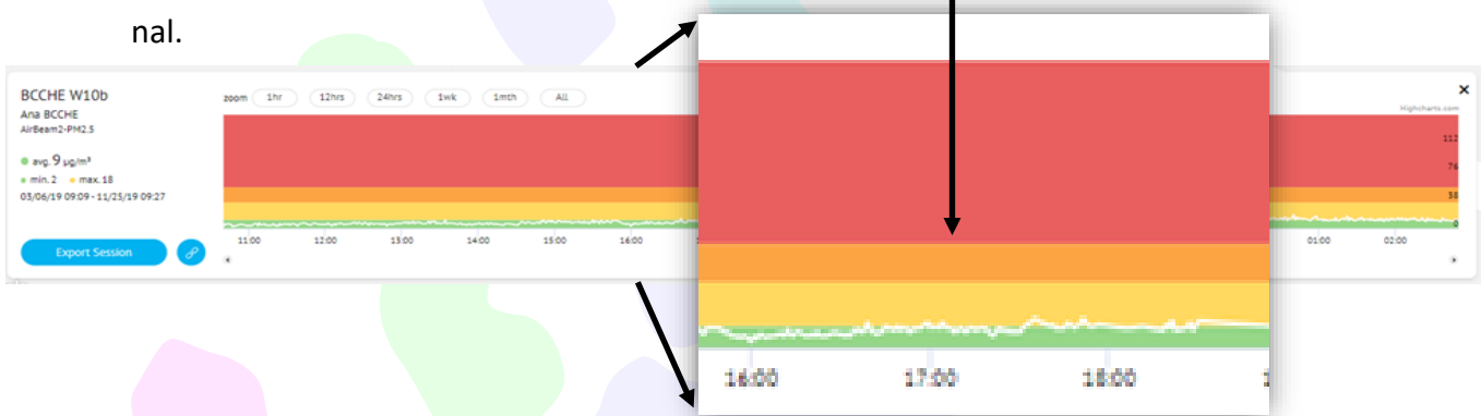
Figure 25. AirBeam2, W10b noise in sensor signal.
