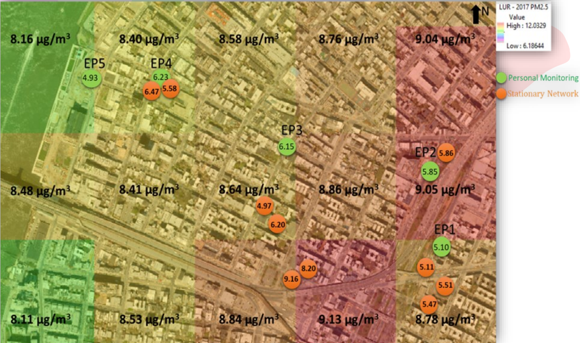
Fig.24. Annual PM 2.5 averages from Land Use Regression (LUR-2017) model along with daily/sessions measurements from AirBeam2, (NYCCAS 2017; Ilie and Eisl, 2019).
